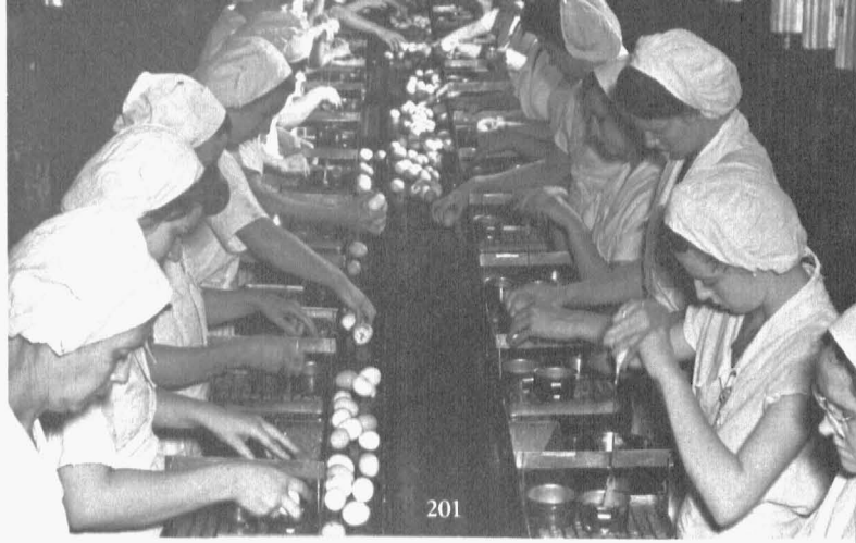
Fig. 204—Battery (10) of egg breaking machines at Tranin Egg Products Co., Kansas City. Liquid goes in stainless steel pipes to holding vats.
