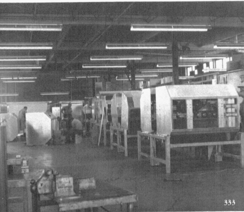
Fig. 331—Assembling poultry packaging machines. Fig. 332—Massive machines are used to shape the stainless steel used in poultry equipment. Fig. 333—Building poultry picking machines. Fig. 334—Packaging machine for cut-up or whole broilers. (Courtesy Gordon Johnson Company, Kansas City) Fig. 335—Poultry processing equipment leaving the factory in Kansas City (Courtesy Gordon Johnson Industries, Kansas City) Fig. 336—Processing equipment in sealed container for export. (Courtesy Gordon Johnson Industries, Kansas City)
