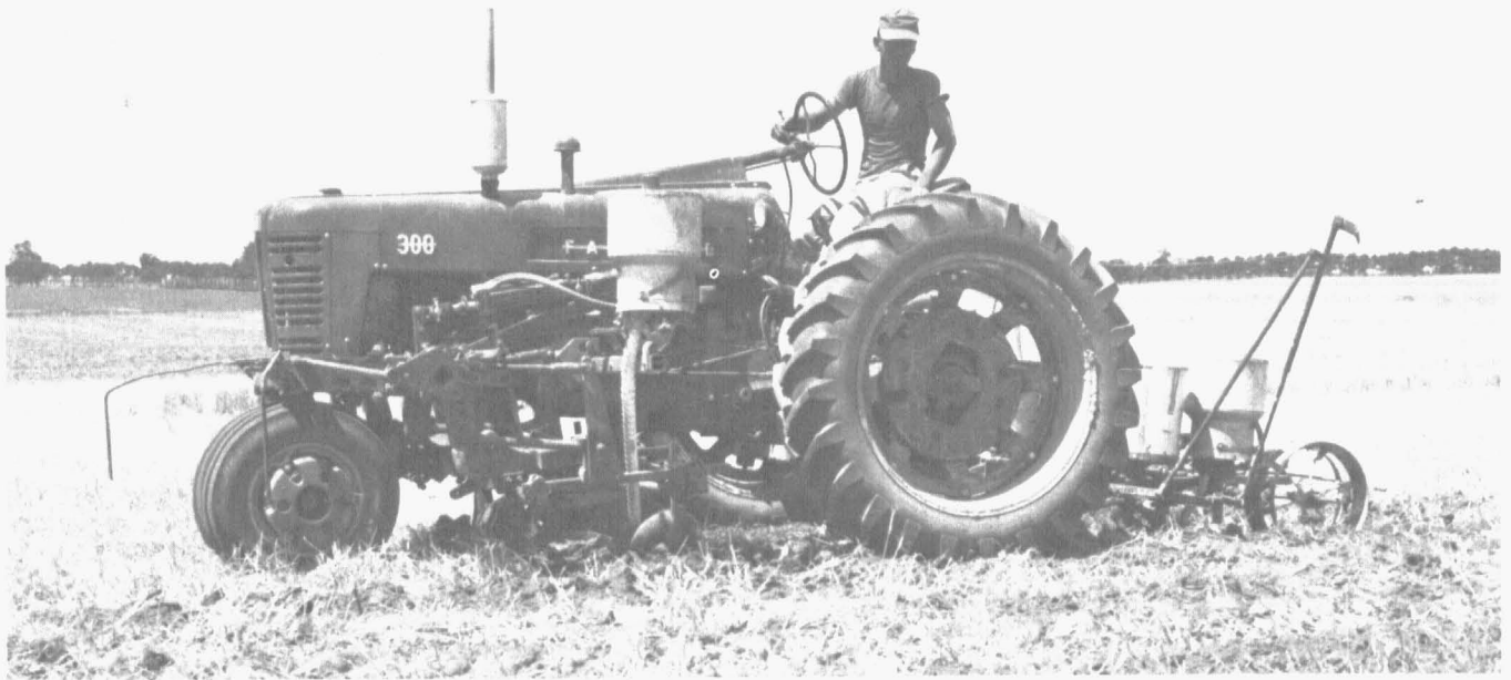
Fig. 1 The once-over strip tilling and planting equipment used in the first experiments on reduced tillage. The strip tiller equipment, mounted on the tractor cultivator frame, consists of wide sweeps to clear trash from the row areas,
