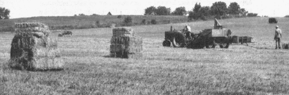
Figs. 6, 7, 8.—The one-man pickup baler saves labor and time. This machinery working under favorable conditions can make at least 100 to 150 bales an hour. Note the slide for piling the bales. When the slide is loaded the pile of bales is pushed off. The piled bales are left in line for easy collection by the wagon.
