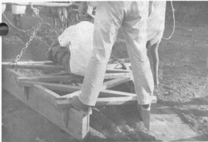
Oxen-drawn border drag made by villagers for building contour borders for surface irrigation.
