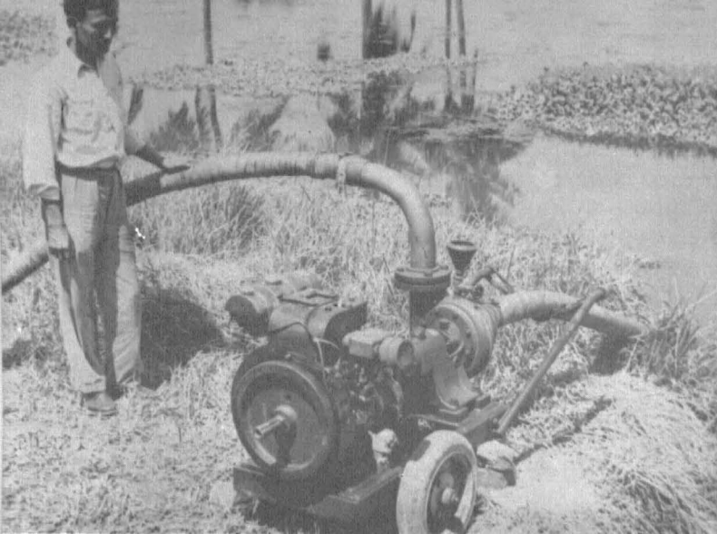
This portable irrigation pump with diesel engine is being used at the college experiment station in Bihar.
