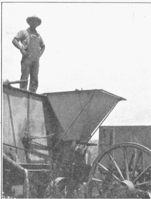
Fig. 2.—Threshing machine attachment for artificial manure production as used on the Poirot Farms.
