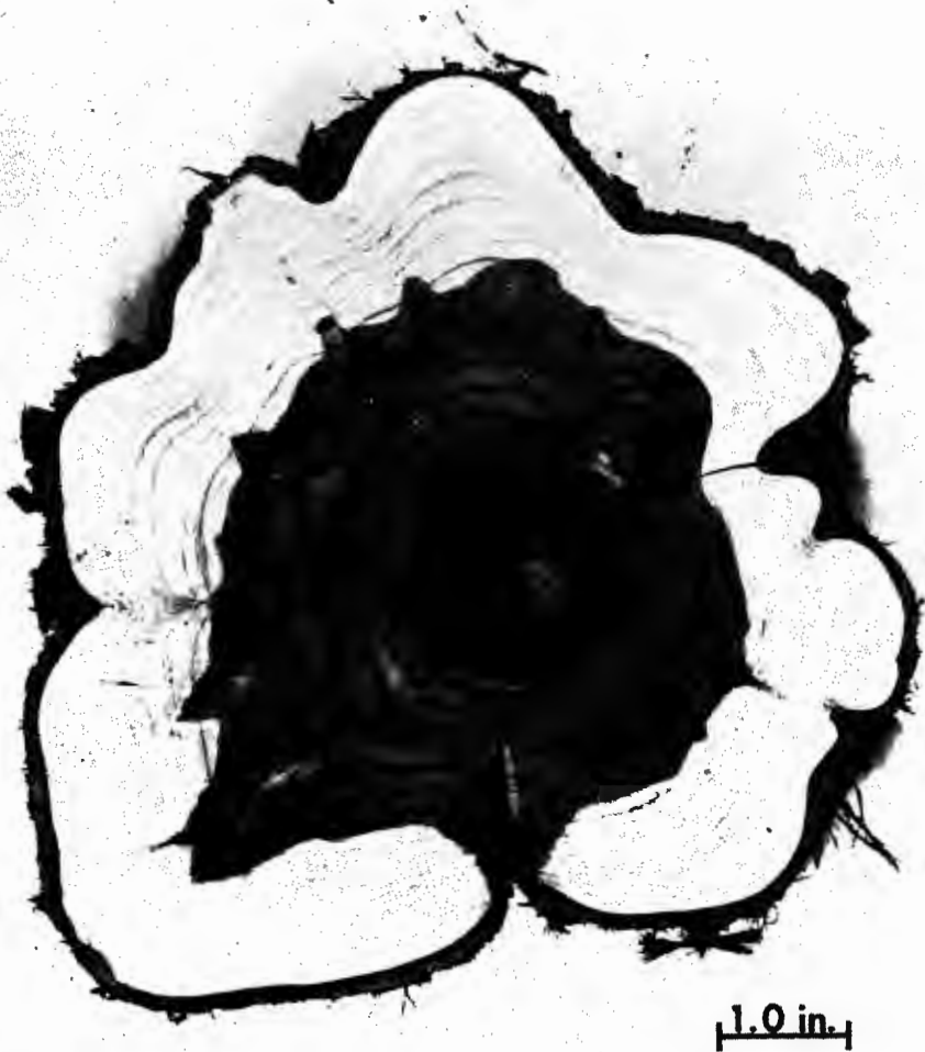
Fig. 9—Cross-section of redcedar. Determination of growth rate is complicated by both the wavy or convolute pattern of growth typical of this species plus the presence of numerous "false" rings formed during the growing season.
