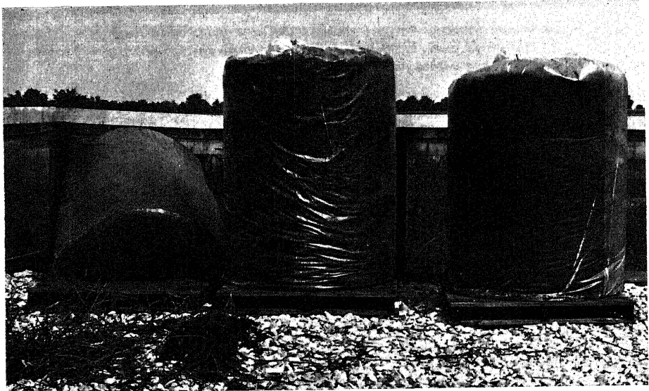
Fig. 11—Bags filled to a depth of 6 ft. with direct cut alfalfa (left) did not remain upright. Bags filled to a depth of 6 ft. with wilted alfalfa (center bag) and to a depth of 5 ft. with direct cut alfalfa (right) did not topple over, although some did lean. The bags are 4 ft. in diameter.
