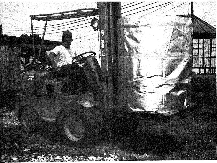
Fig. 18—The bags, 4 feet in diameter and 5 feet tall, were handled by a fork lift. The bags held approximately 1200 pounds of chopped alfalfa.
