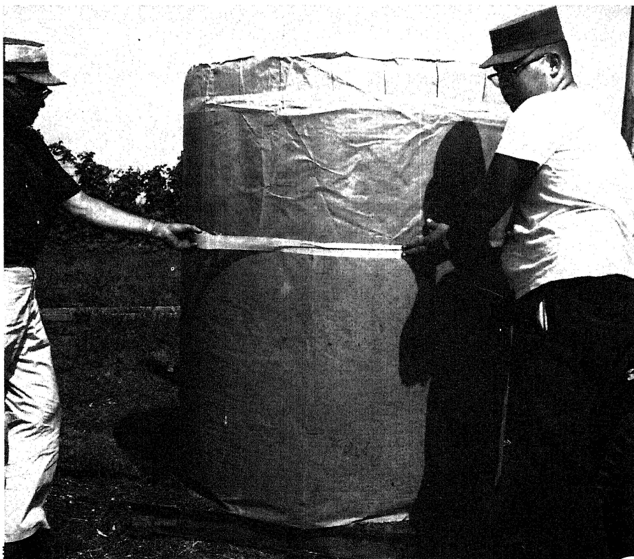
Fig. 17—The cap was sealed in place with three layers of masking tape.
