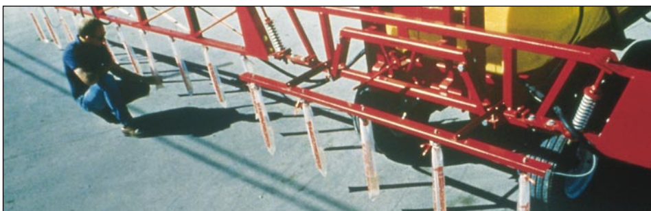
Check individual nozzles separately and calibrate sprayers to maintain accuracy.
