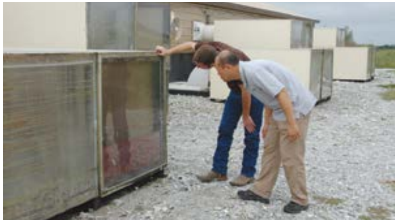
▲ MU Extension assistant professor Teng Lim and graduate assistant Brandon Harvey examine the material inside a biofilter at the MU Swine Research Center. Lim's research centers on management systems to minimize odor, dust and gas from swine operations.
