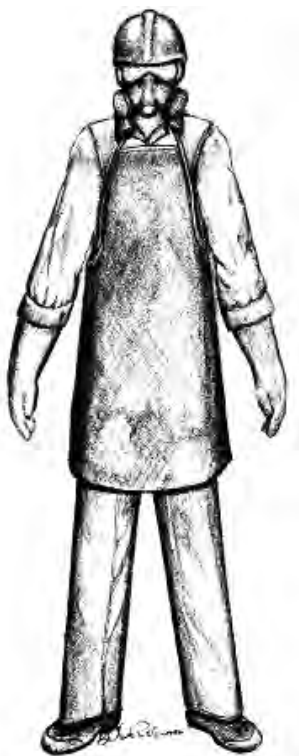
Figure 22. Proper attire for a worker entering the area around the treatment cylinder door.
