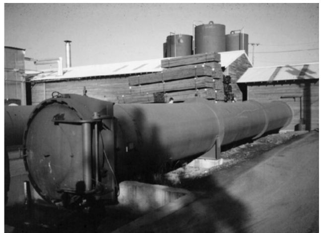
Figure 14. Example of a pressure treating facility showing a retort as well as storage tanks in the background.
