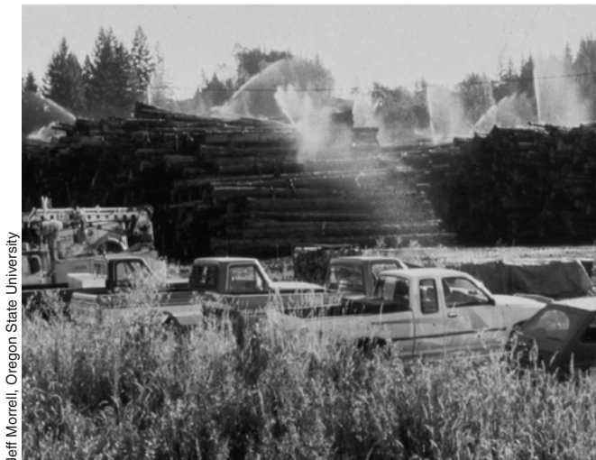
Figure 4. Logs being sprayed with water to limit biological attack.
