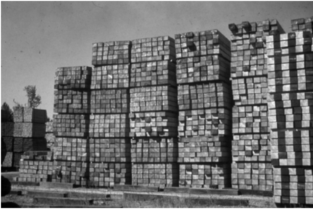
Figure 15. A well laid out air-seasoning area should be free of vegetation with graveled areas, wood off the ground, no woody debris and spacing that allows for even airflow to facilitate drying.
