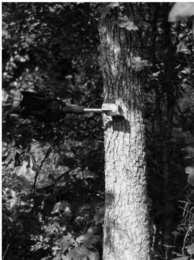
Figure 3.14. The hatchet injector delivers metered amounts of undiluted herbicide directly into the sapwood of the target tree. Credit: James H. Miller, USDA Forest Service, Bugwood.org.
