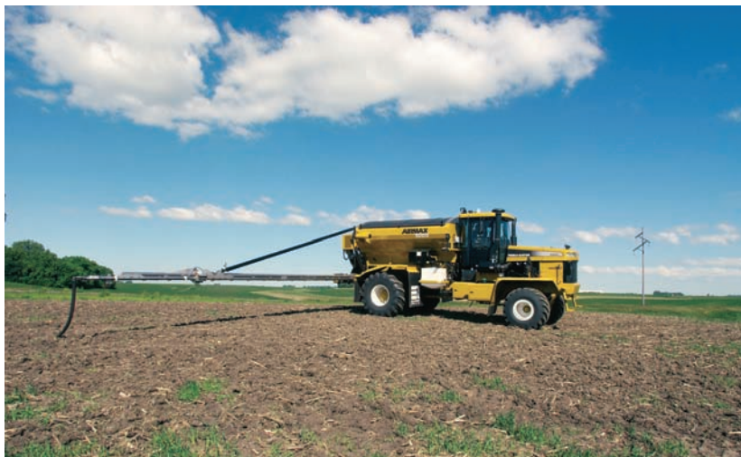
Figure 5. Broadcast applications are suitable for ammonium nitrate, for urea that has been treated with Agrotain or that will be tilled in, and for N solution applied in low-residue fields. Boom spreaders often give more even application than spinner spreaders.
