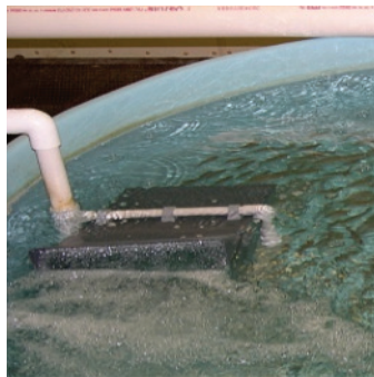
Figure 6. Manifold aerators not only provide oxygen but also create a circular flow that aids in waste removal.
