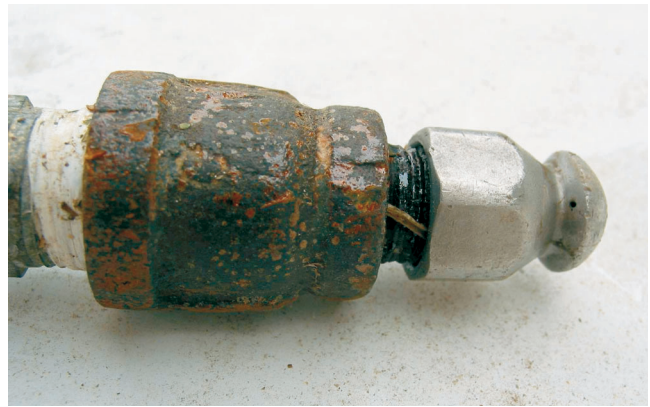
Figure 5. This sewer nozzle is made of stainless steel for long-term durability.
