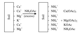
The potassium concentration in the ammonium acetate soil extract is determined by flame emission. The extract sample is sucked
