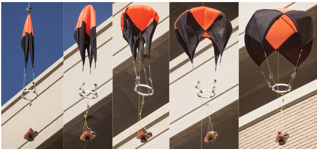
Figure 8: Inflation sequence during a zero-length static line deployment.
