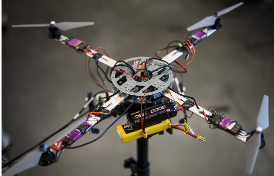
Figure 12: Constructed quadcopter with instrumented arms mounted onto load cell test stand.
