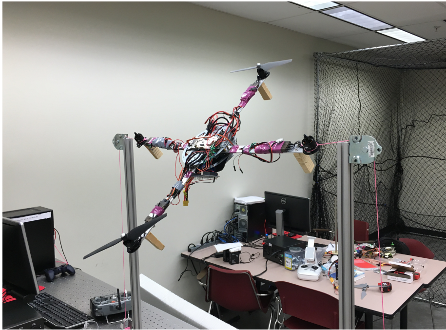
Figure 21: Single axis constrained full motor failure test setup
