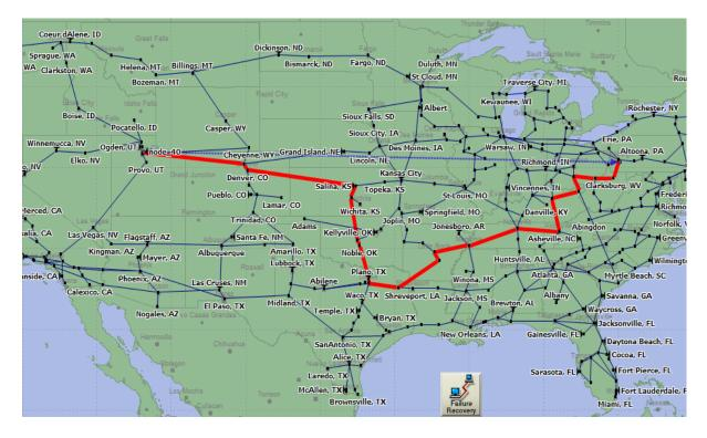
Figure 61: Single Demand Using Selected Topology Routing based on gMTR
