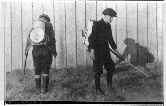
Fig. 17.—Bellows type dusters for applying dust mixtures on potatoes or other garden crops.
