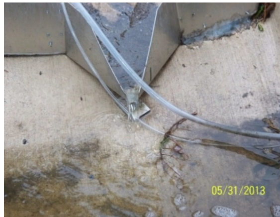
Figure 18 0.5H Flume Inlet
