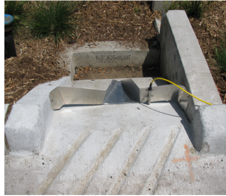
Figure 15 Global Water Level Sensor
