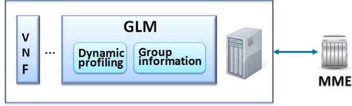
Figure 10: Virtualized network function for group location management
