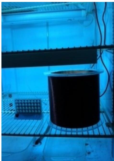
Figure 12. Experimental set-up for cycles of magnetism. A magnetic field was produced inside a solenoid by passing an electric current through the coil, with the strength of the field being proportional to the current. A DC power supply on a timer (12hr on:12 hr off cycles) was used to generate current through the solenoid. Light was produced by high intensity blue fluorescent bulbs in the incubator with wavelengths ranging between 450 nm and 470nm.
