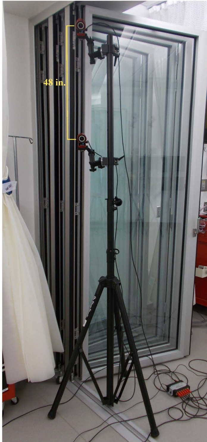
Figure A.1. Setup of Two Flex 13 Cameras Mounted Onto an On Stage Stand
