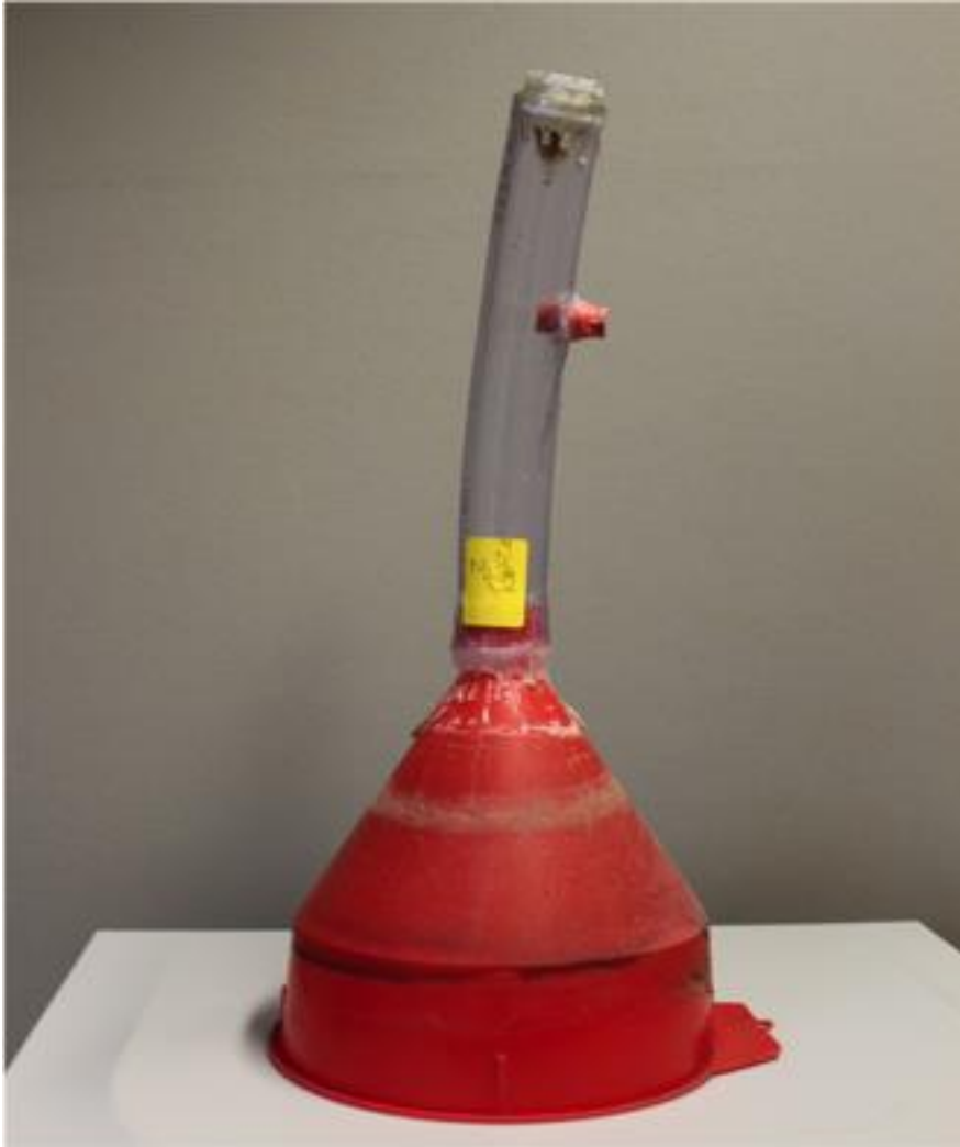
Figure 2.1 A static chamber used to collect gas samples for GHG emission analysis.
