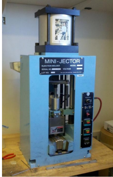
Fig. 2.2. Digital camera image of Mini-Jector used for injection molding. Machinery Corporation, Newbury Ohio.
