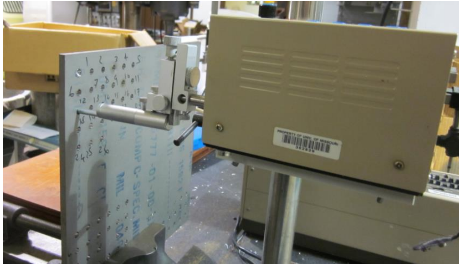
Figure 2-10: Setup of the surface roughness measurement
