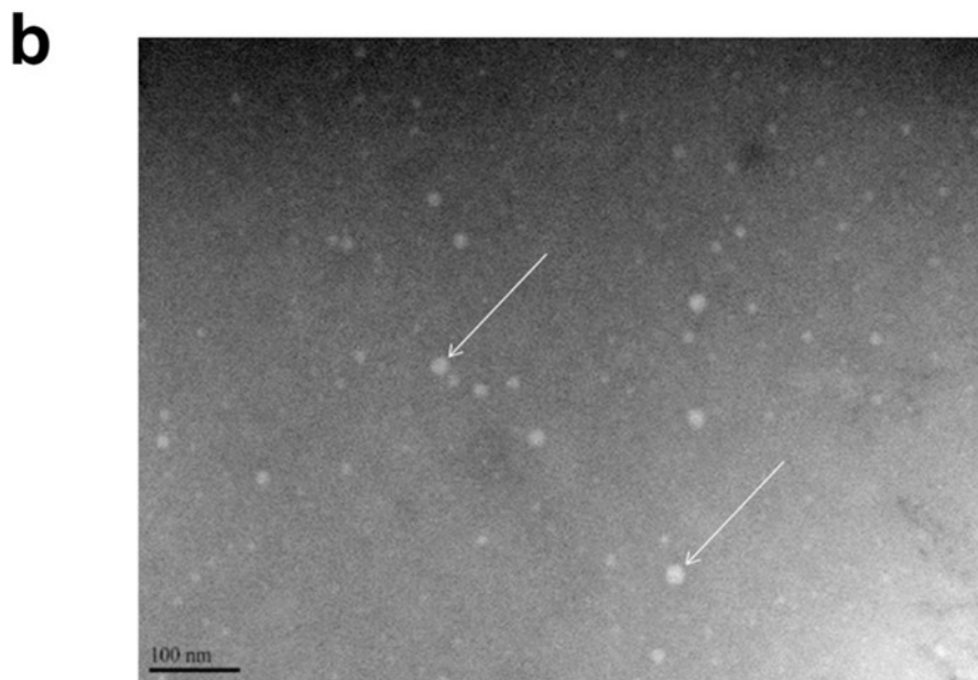
Figure 4-9 (a) Micelles size distribution for DEXM for design run #2 of ED-2. (b) Transmission electron micrograph for DEXM. Nanomicelles appear as a white spot on dark background as indicated by arrows.
