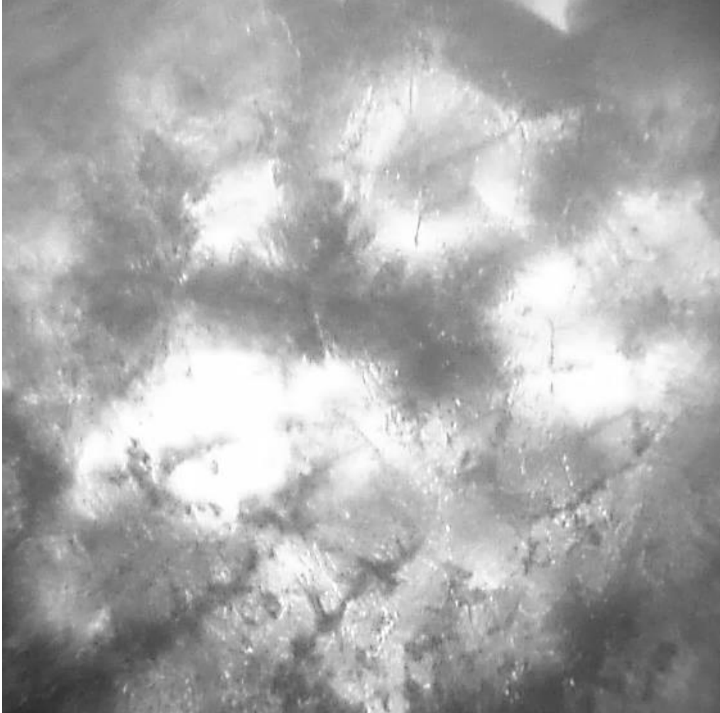
Figure 35: Run 54 optical image at 400x magnification. Glassy, transparent surface allows light to pass through showing the polycrystalline structure underneath.
