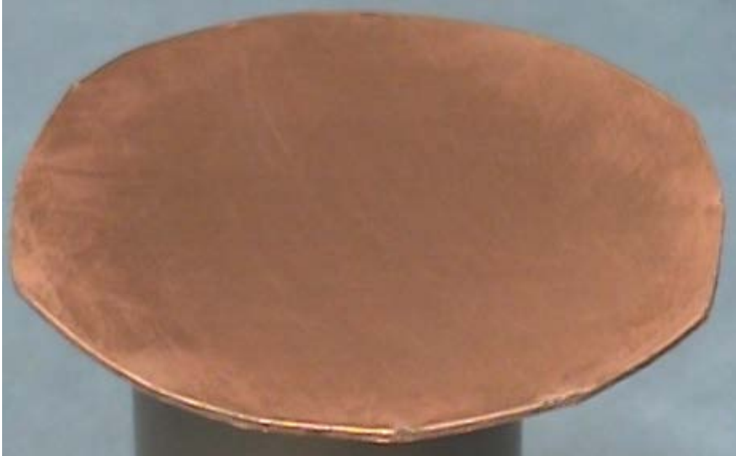
Figure 78: Brush on nano-diamond technique macro image on copper
