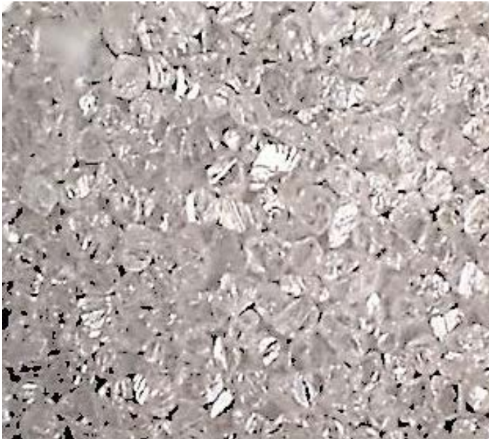
Figure 8: Aligned diamond crystals before HFCVD run. Open area was determined using Adobe Photoshop® analysis package. Calculated open area is shown as black. Magnification is 400x.
