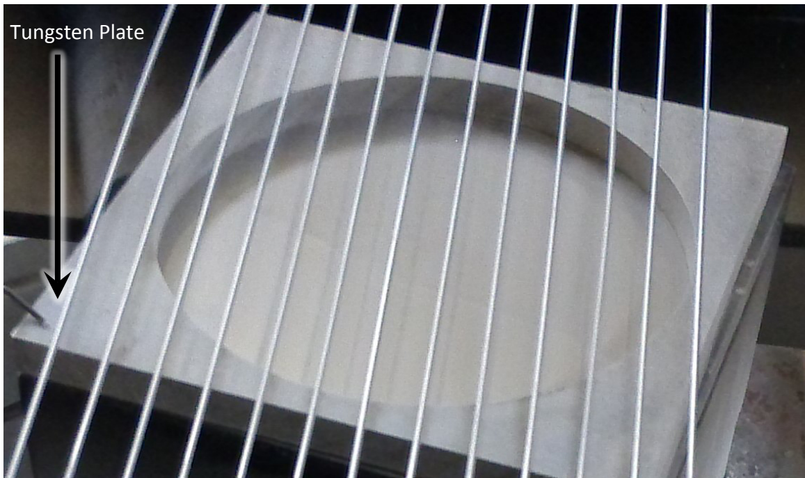
Figure 63: Run 64 shown with tungsten plate and platinum substrate holder.
