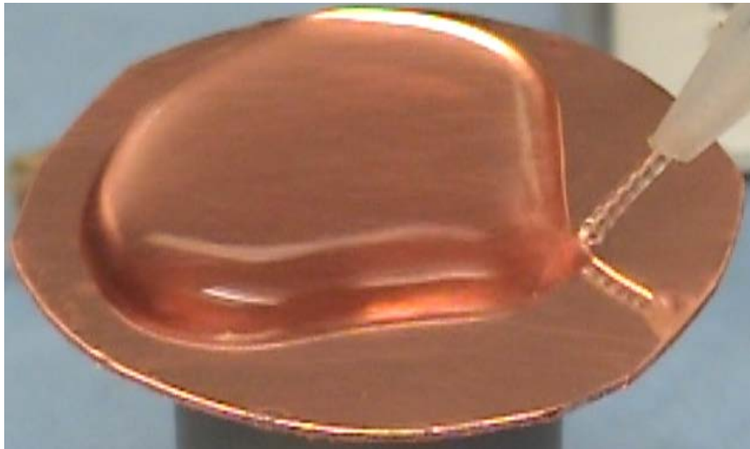
Figure 72: Without Nano-Diamond Pretreatment: Application of DI water on a copper surface. High surface tension and low adhesion creates a near 90 degree angle between the copper and water
