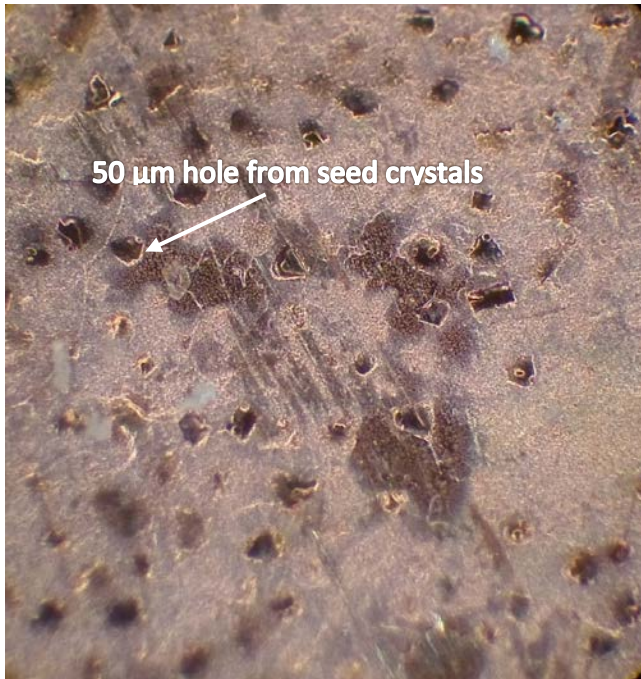
Figure 12: Run 4a. Optical microscope image of diamond film growth on copper. Holes that appear in the image are a result of 50 µm seed crystals that came off during reactor shut down.
