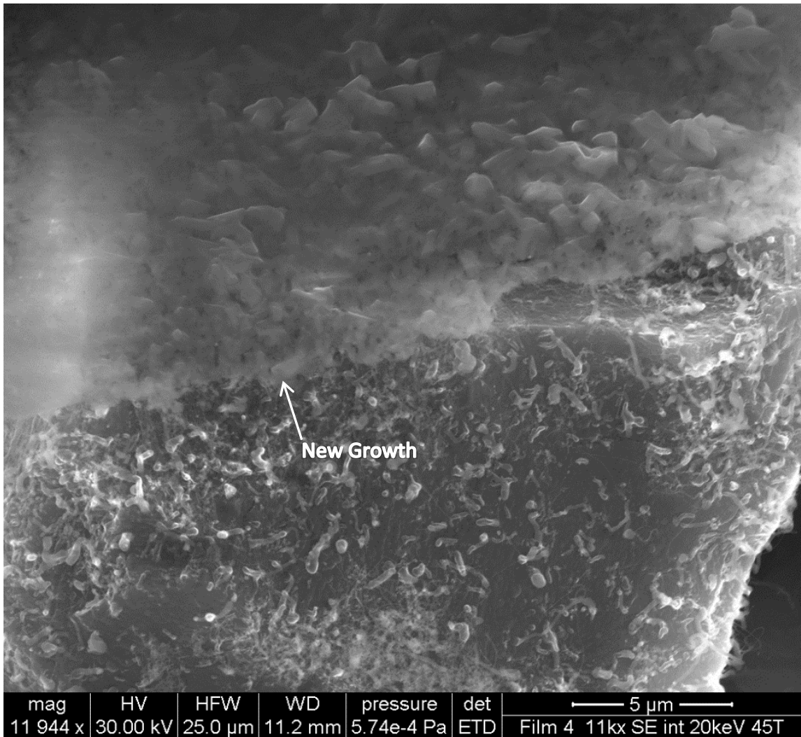
Figure 17: Run 6. Close-up of a single 50 μm seed crystal shown from the side. Top portion of the crystal is new growth.
