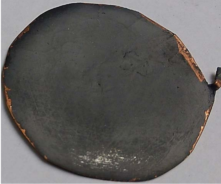
Figure 28: Run 47. Diamond Like Carbon (DLC)/diamond (111) growth bonded to copper. The film cannot be scratched (even with diamond) or removed from the copper.
