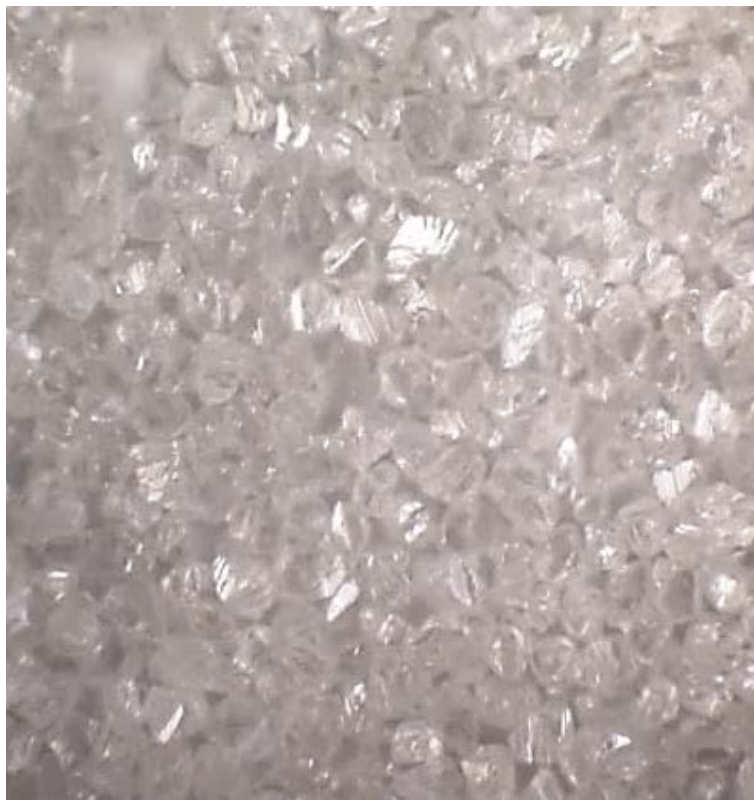
Figure 76: alignment final result. A single layer of crystals deposited on top of a metal holder. Crystals shown are 50\ \mu\text{m} \pm 10\%
