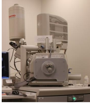
Figure A1.4. Scanning electron microscope (SEM Quanta) used to image the fracture surface of HA/PLA composite.
