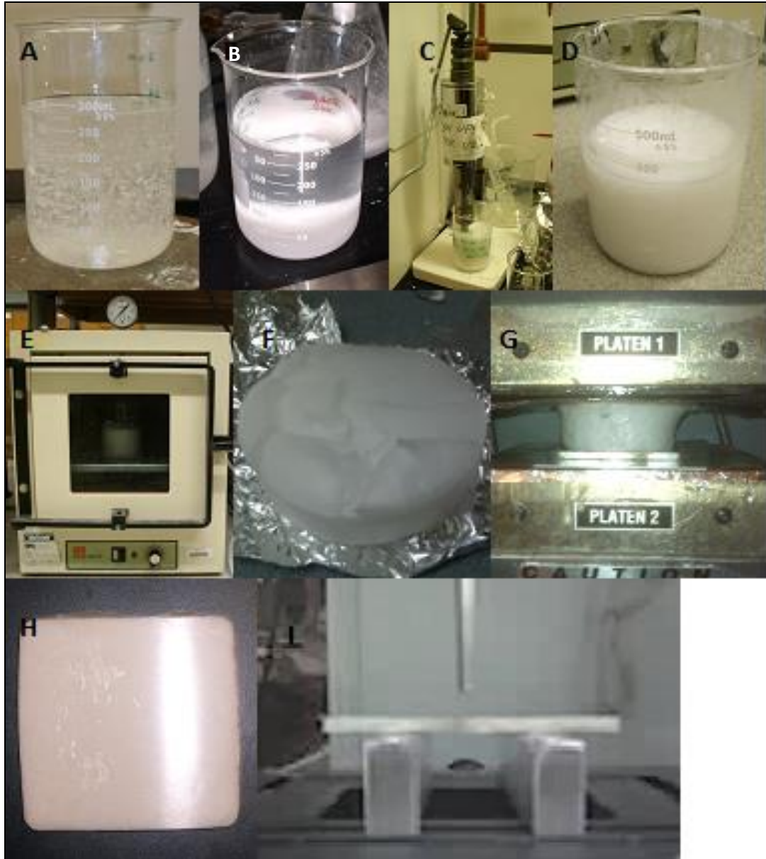
Figure.A1.2. The complete hot pressing procedure:(A) pure PLA pellets and methylene chloride solution are first added; (B) pellets are completely dissolved in methylene chloride solution (C) HA is mixed with PLA using ultra-sonic horn and mechanical assistance (D) methylene chloride solvent forms an HA/PLA solution (E) Methylene chloride is evaporated using a vacuum oven (F) from vacuum oven HA/PLA emerges as a composite disk (G) Hot pressing procedure yields (H) mold removal and (I) samples are cut and tested under three point bending on an universal texture analyzer.
