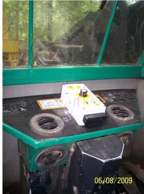
Figure 5. Yellow Activity Monitoring System data collector “Yellow Box” attached to skidder
