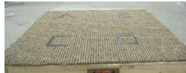
Figure 1: Development board carpet is atop a wooden frame (made up of 5cm X 10 cm, i.e. 2 X 4 studs) approximately 1 m X 1 m. The four sensors are under the carpet; wires come through the wooden frame and attach to the circuit board shown
