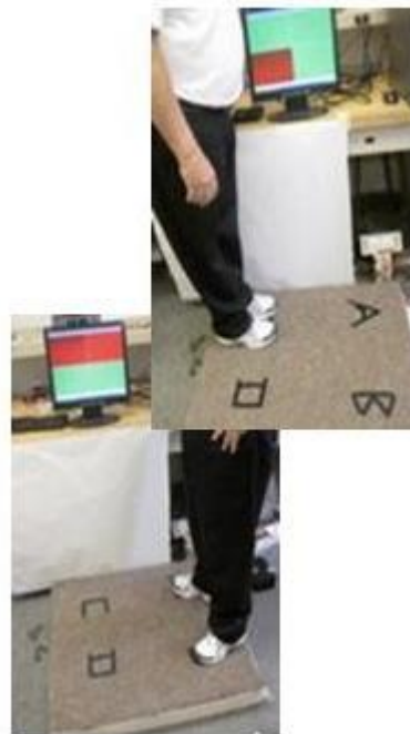
Figure 3: Person standing on the carpet activating sensor C (upper) and both sensors A and B (lower). The green background LCD displays the activated sensor in red. Note the red screen quartile in the lower left quarter of the display of the upper figure. Similarly the activation of A and B causes the lower half of the screen to turn red.
