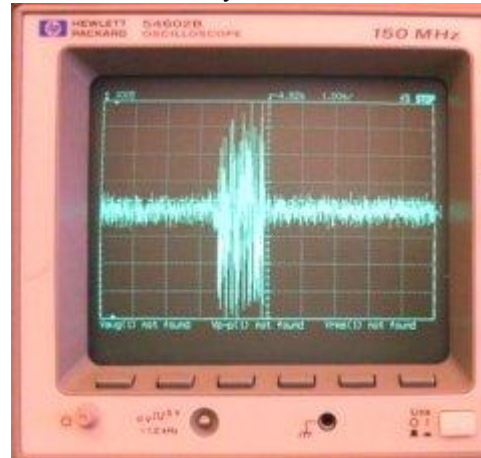
Figure 3 Electrical energy added to the foil as a result of a person touching (activating) the foil. The smaller noisy portion of the trace has a level at 30mv p-p, whereas the larger activated portion is nearly half a volt.
