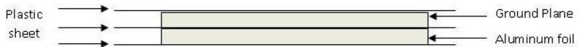
Figure 3.1: Arrangement of the 2x2 Development System layers. Plastic sheet covered the wooden base followed by ground plane, plastic sheet and finally the sensor layer.
