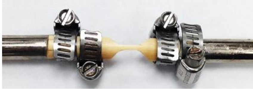
Figure 2-2 “Dog-bone” shape specimen.
