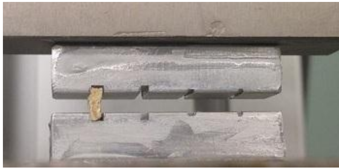
Figure 2-5 Specimen preparation for compressive test on transversal direction .
