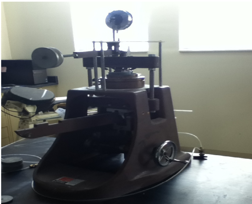
Figure A.36 Incremental load test apparatus.
