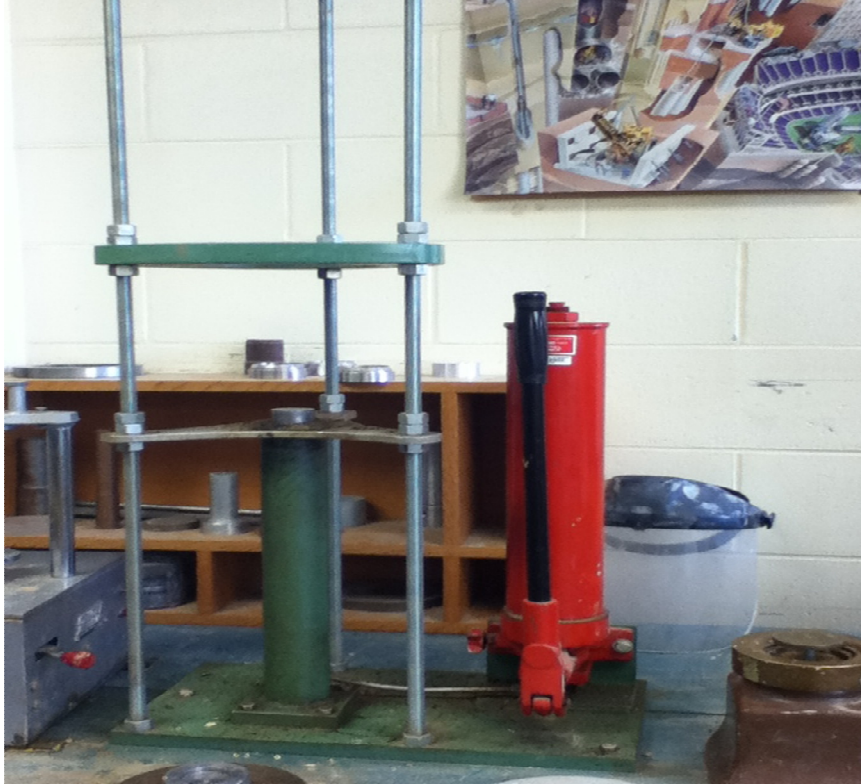
Figure A.35 Extractor device used for extracting specimen from Proctor mold.
