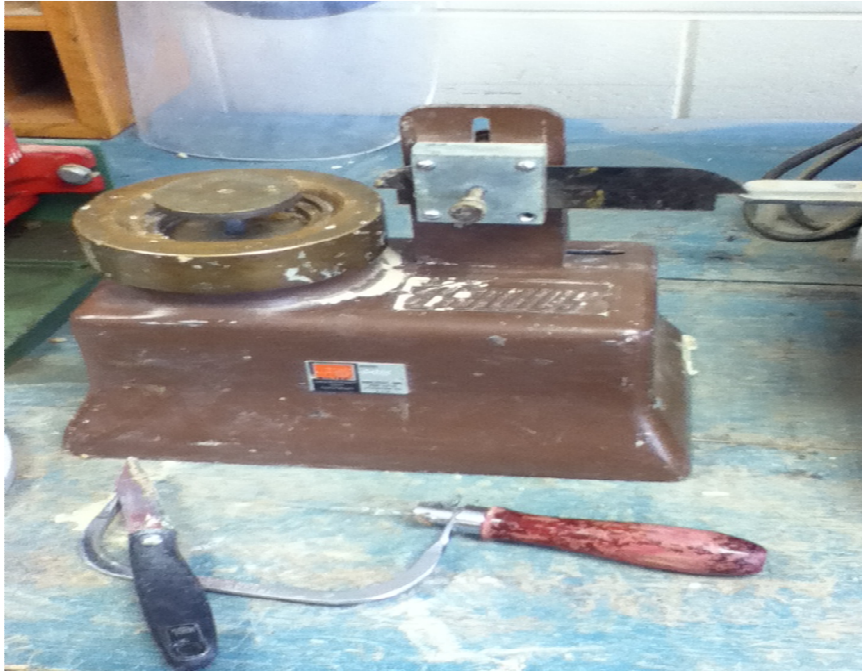
Figure A.37 Trimming tools used for preparing FGD sludge specimen.
