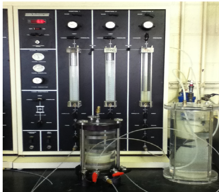
Figure 3.4 Permeability apparatus in MU geotechnical engineering laboratory.
