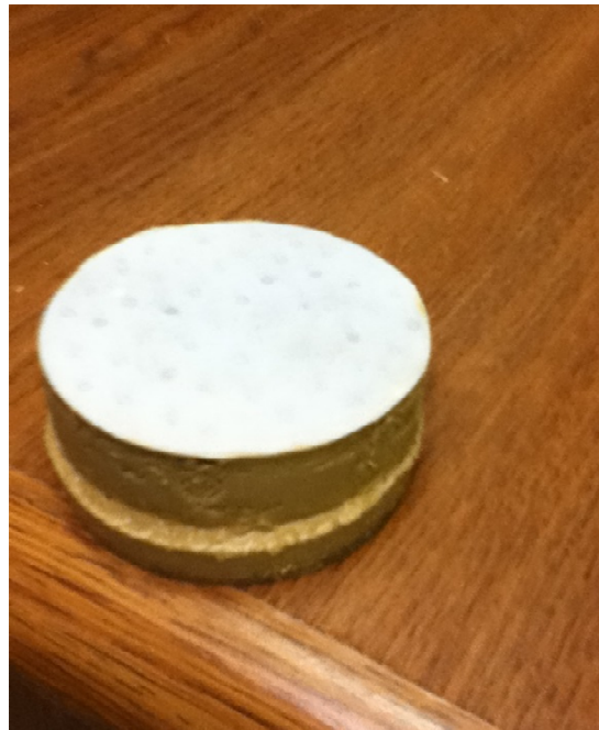
Figure A.34 Plan view of failed compacted FGD specimen after test.
