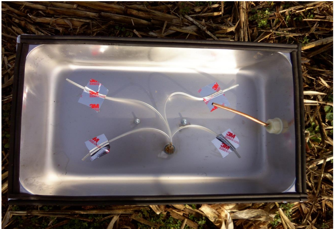
Image 2-2. Chamber used to collect GHG emissions, viewed from the inside.
