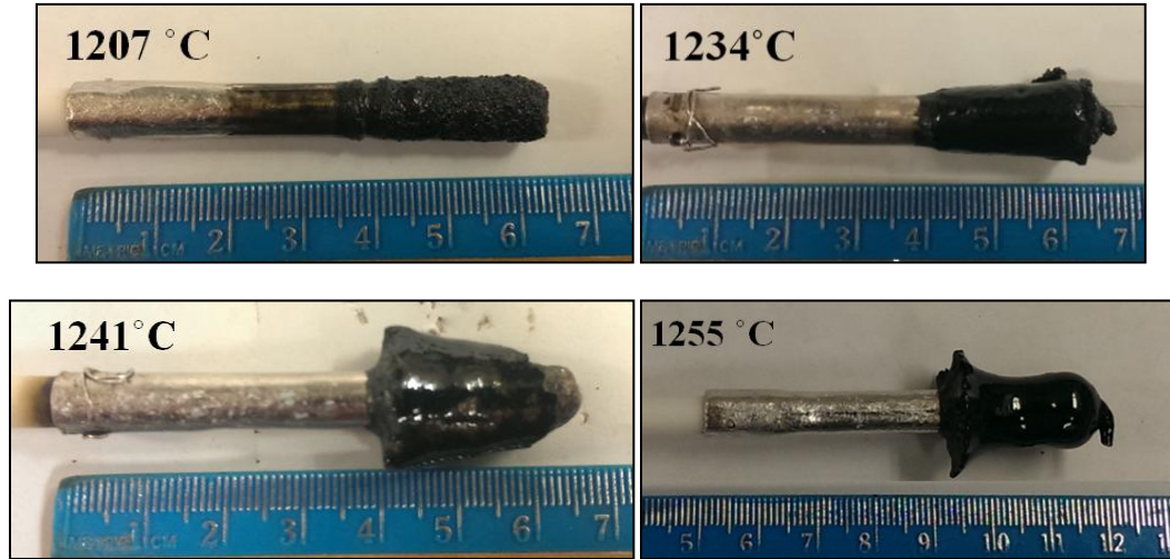
Figure 3.13. Melt accumulation on spindles, yielding artificially high stress values.
