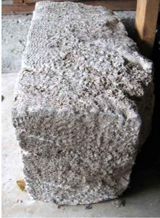
Fig. 4 Showing chiseled stone and uneven fracture along the back
