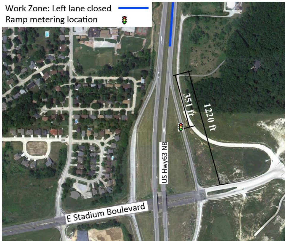
FIGURE 3.13 Work zone layout on US-63NB @ Stadium, left lane closed.
