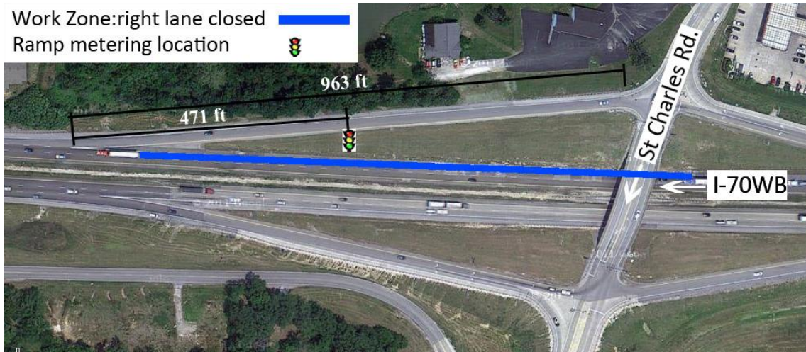
FIGURE 3.4 Work zone layout, I-70WB @ mile marker 131.
