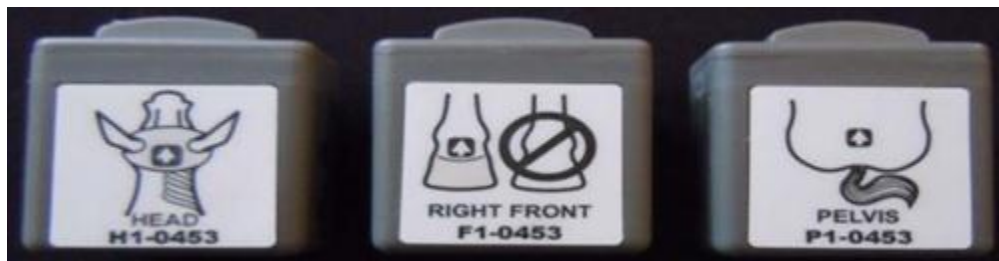
Figure 1.5: A wireless gyroscope (middle) and two wireless accelerometers [2].
