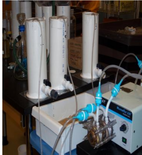
Figure 3- 2: General Setup used in All Tests of PVC Column and Associated Equipment Setup of Bioretention Cells: BSM + Water Treatment Residuals
