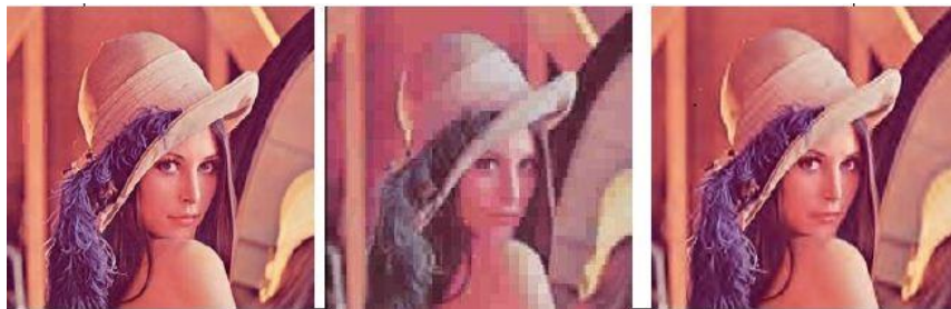
Figure 36 JPEG2000 perform better than JPEG in lower bit rates (left: original image; middle: JPEG right:JPEG2000)
