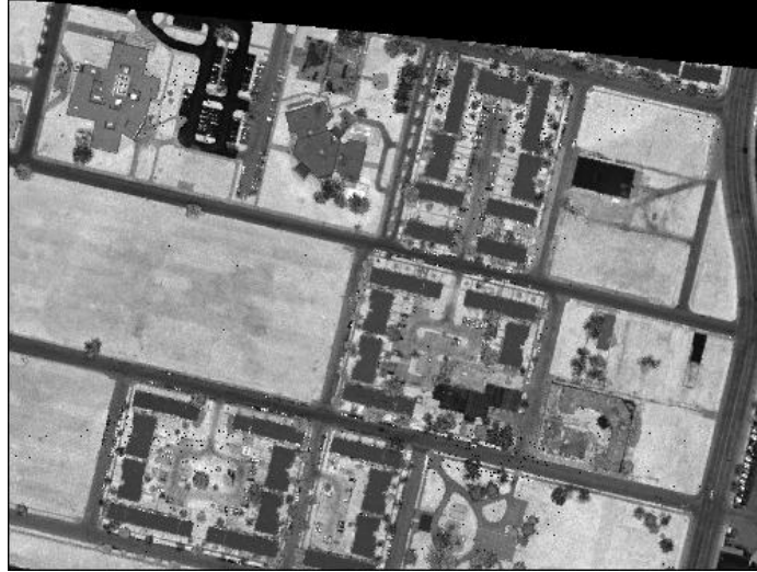
Figure 14. This is a visual display of laser returned intensity.
