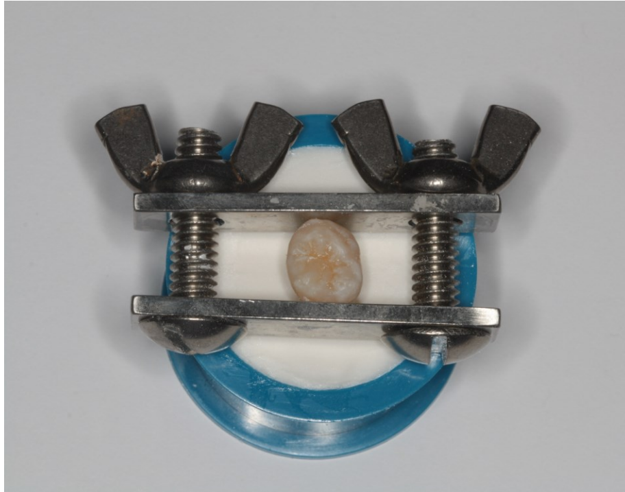
Figure 1. Maxillary third molar embedded in self-cure acrylic resin.
