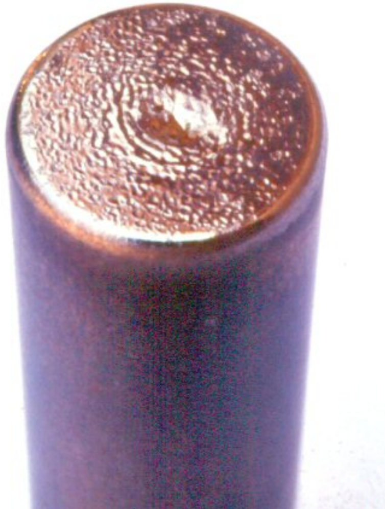
Ti Anode of PF Device after 50 shots
