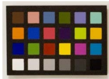
Figure 2: Image of a GretagMacbeth Mini Color Checker, which is the one used in all our experiments.
