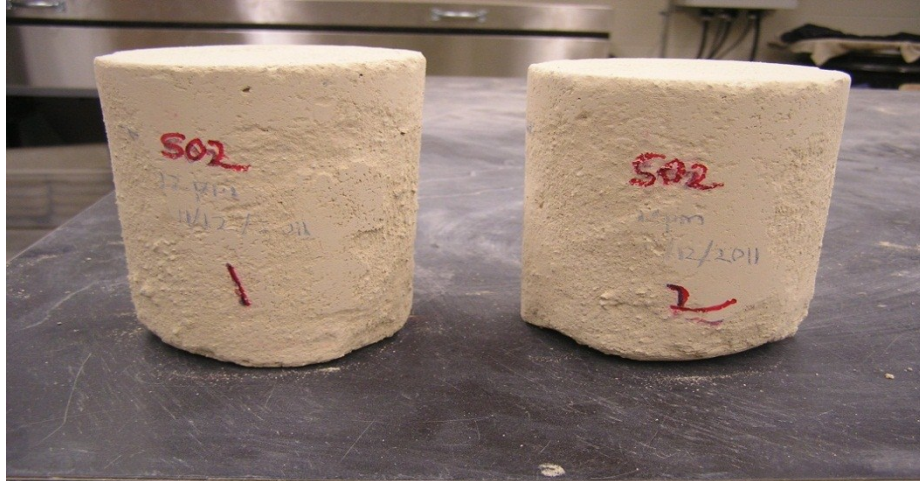
Figure B5. Unsaturated samples S02 after 11 freeze-thaw cycles
