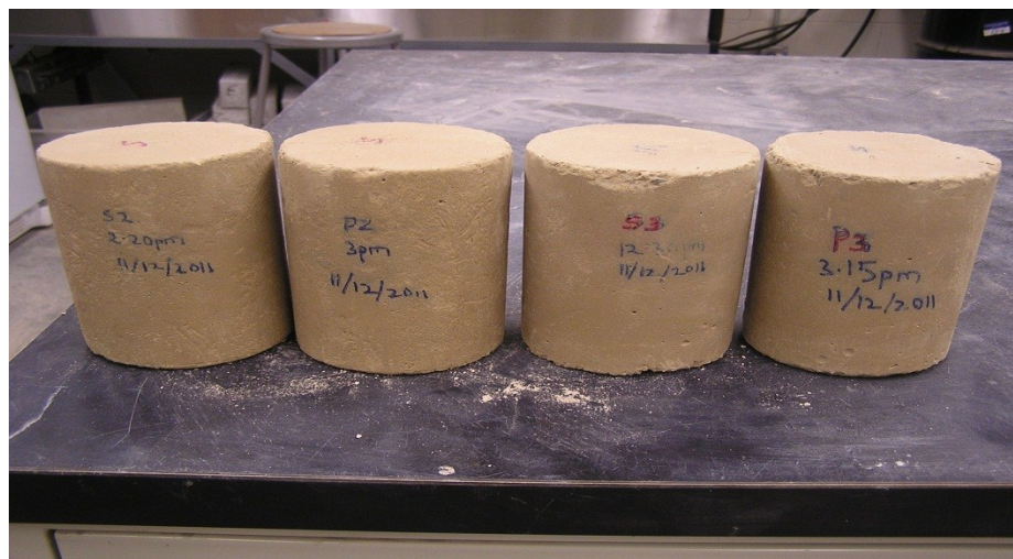
Figure B10. Saturated samples S2, P2, S3, and P3 after 11 freeze-thaw cycles
