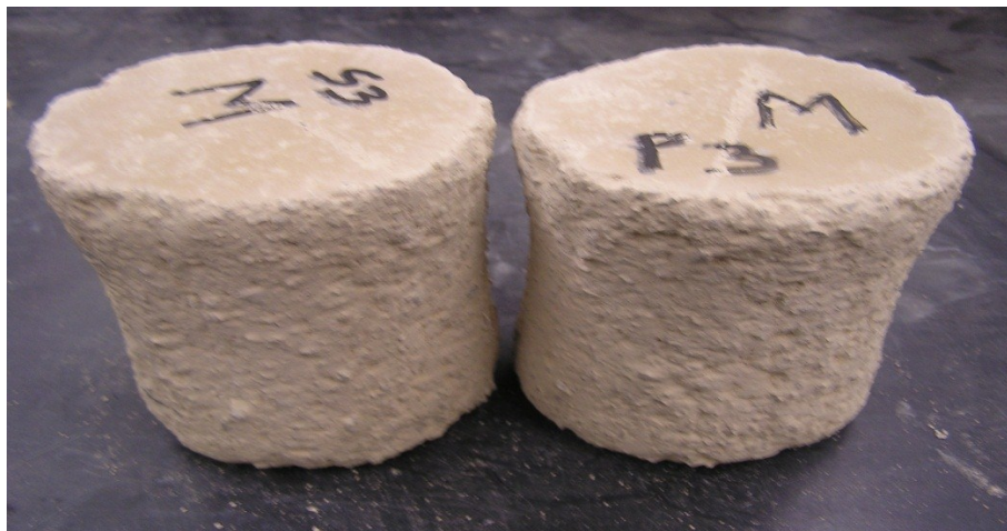
Figure A4. Saturated samples S3 and P3 after 36 freeze-thaw cycles
