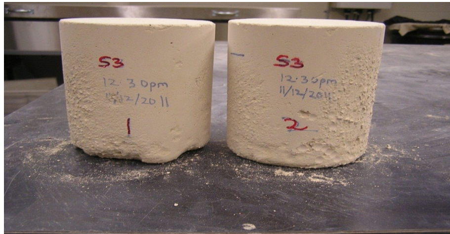
Figure B8. Unsaturated samples S3 after 11 freeze-thaw cycles
