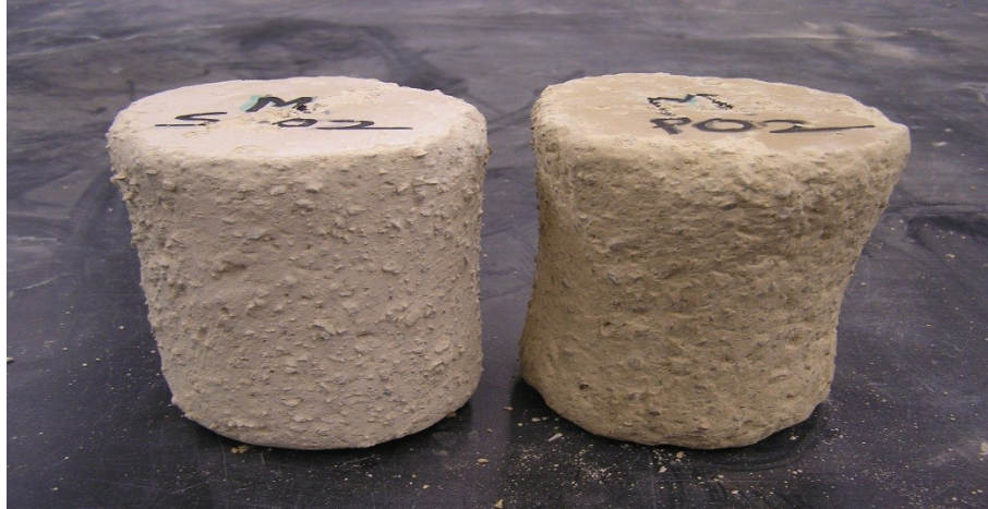
Figure A3. Saturated samples S02 and P02 after 36 freeze-thaw cycles
