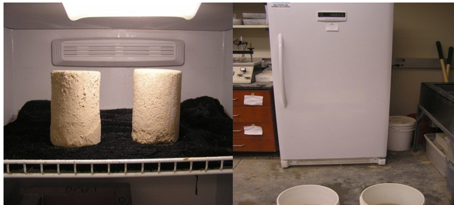
Figure 3-9: Set up for freezing of samples
