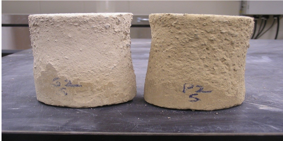
Figure B17. Saturated samples S2 and P2 after 44 freeze-thaw cycles
