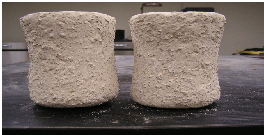
Figure 3-12: Samples with Sunflower quarry fines (left) and Parkville quarry fines (right) after 44 freeze-thaw cycles (20 % gypsum by weight of fly ash and W/FA ratio of 0.8)
