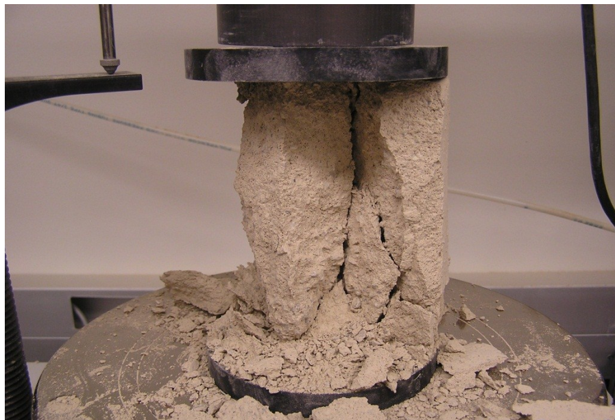
Figure B22. Testing for unconfined compressive stress after subjecting the samples to 12 freeze-thaw cycles
