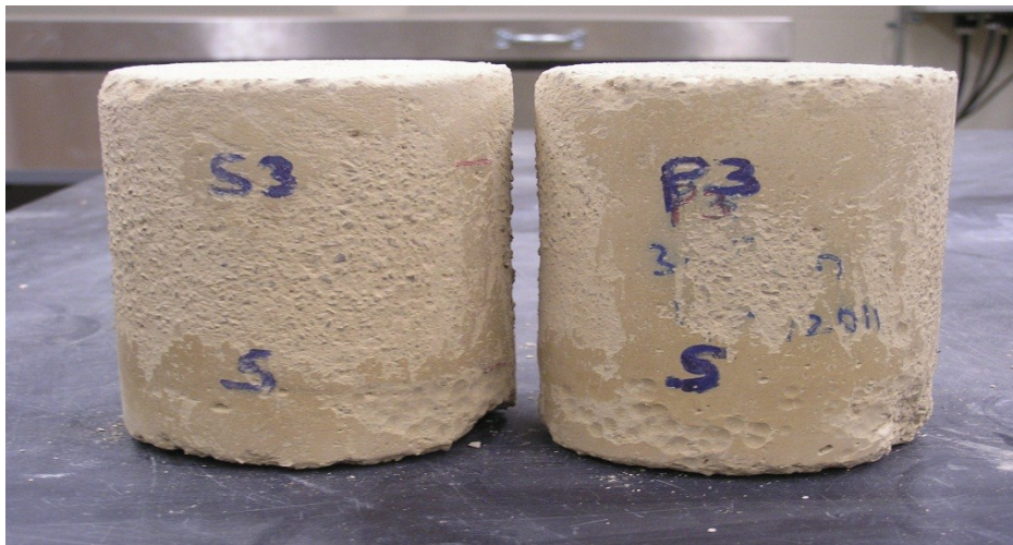
Figure B18. Saturated samples S3 and P3 after 44 freeze-thaw cycles
