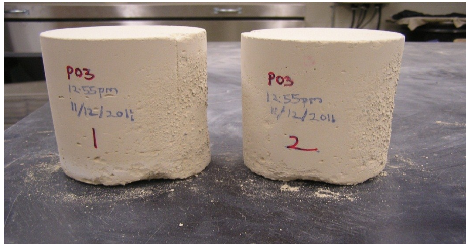
Figure B6. Unsaturated samples P03 after 11 freeze-thaw cycles
