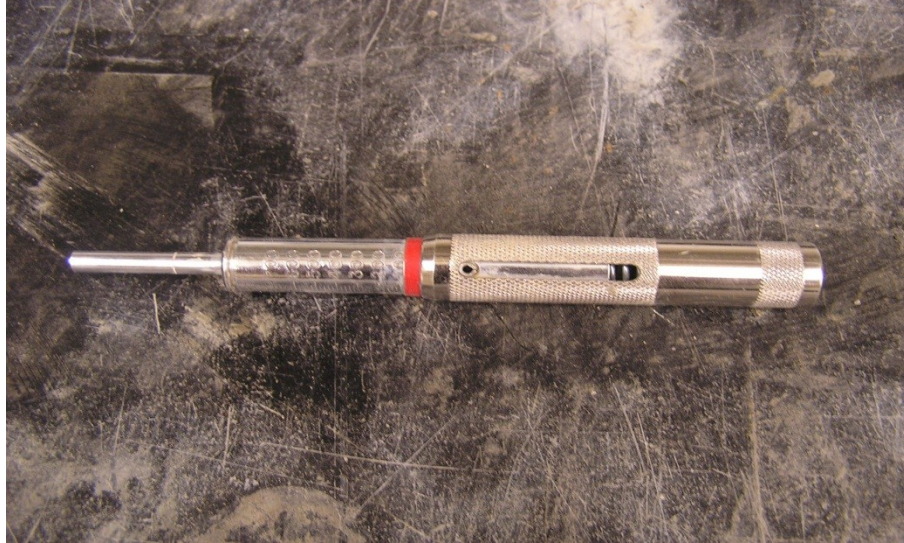
Figure 3-4: A typical vane shear tester
