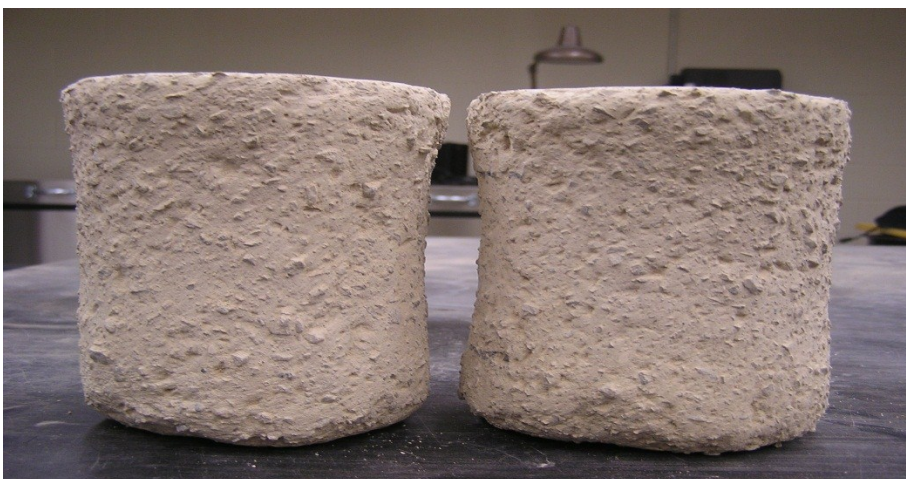
Figure A5. Saturated samples S3 and P3 after 44 freeze-thaw cycles
