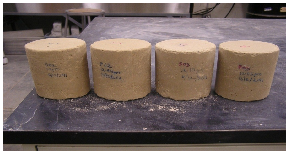
Figure B9. Saturated samples S02, P02, S03, and P03 after 11 freeze-thaw cycles
