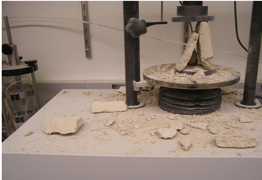
Figure B20. Testing for 56-day unconfined compressive stress after subjecting the samples to 12 freeze-thaw cycles
