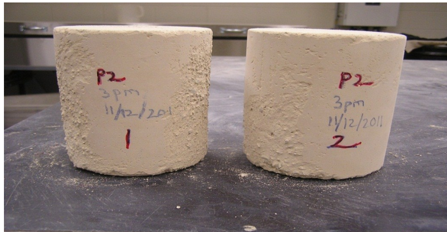
Figure B7. Unsaturated Samples P2 after 11 freeze-thaw cycles
