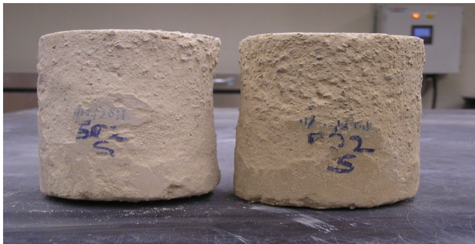
Figure B15. Saturated samples S02 and P02 after 44 freeze-thaw cycles
