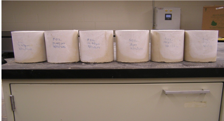
Figure B1. Samples S02 and P02 after 28-days of curing
