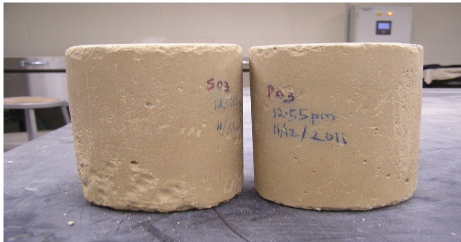
Figure B12. Saturated samples S03 and P03 after 27 freeze-thaw cycles
