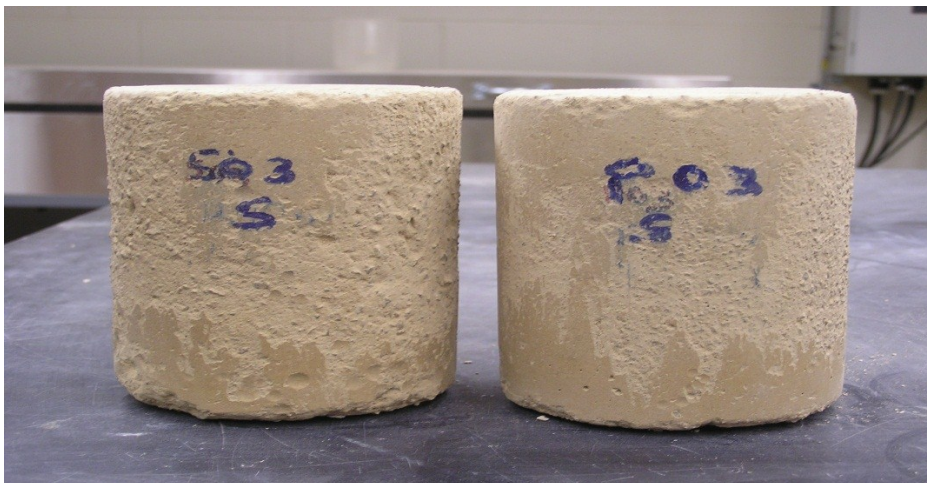
Figure B16. Saturated samples S03 and P03 after 44 freeze-thaw cycles
