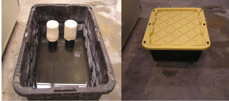
Figure 3-10: Set up for thawing of samples
