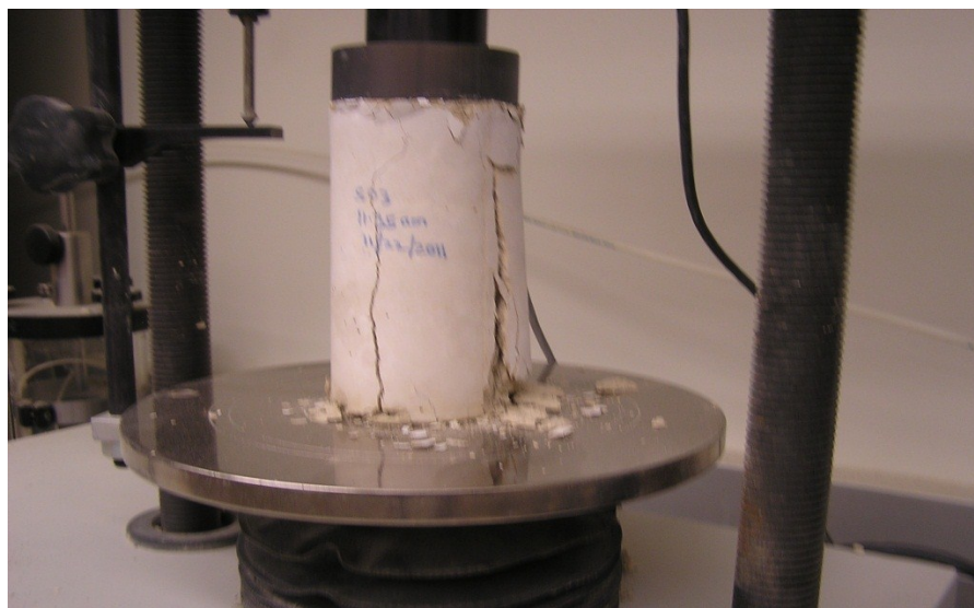
Figure 3-7: Testing for unconfined compressive stress
