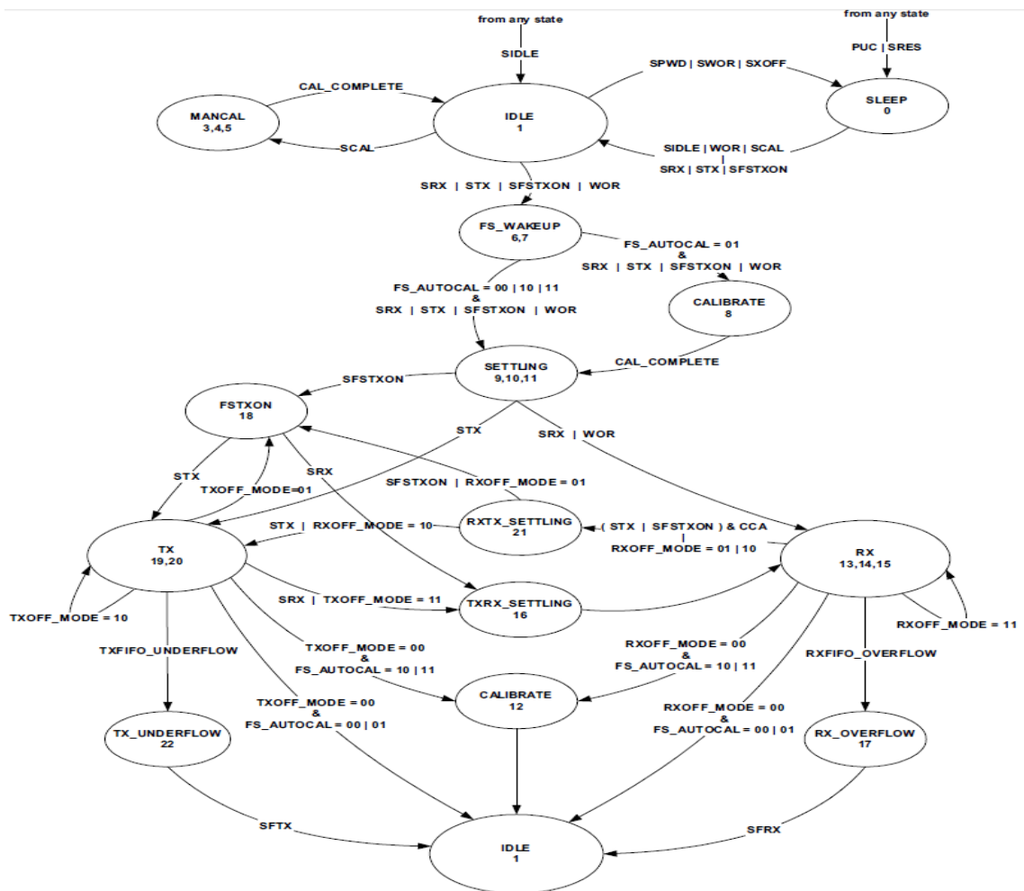
Figure 13: Complete Radio-Control State Diagram
