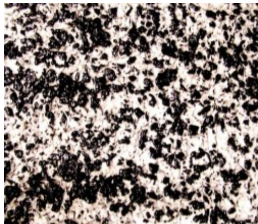
Figure 8: Pervious concrete contact area
