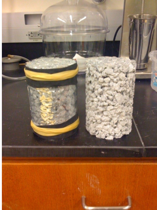
Figure 6: PC cylinders being prepared for permeability testing
