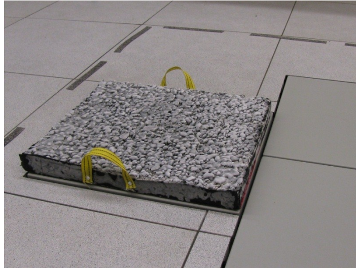
Figure 5: Pervious concrete slab covered with layer of ice atop force platform
