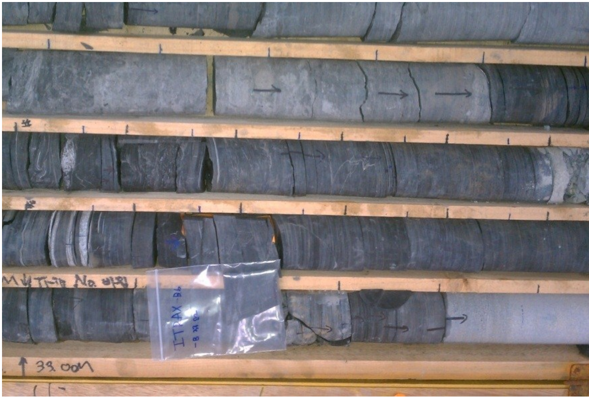
Figure 4.2, Photo of core showing the darker-gray mudstone and lighter-gray sandstone
