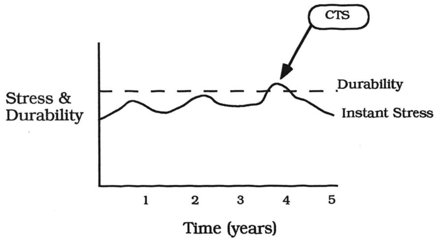
Figure 3.2 Instance stress excessiveness over durability
