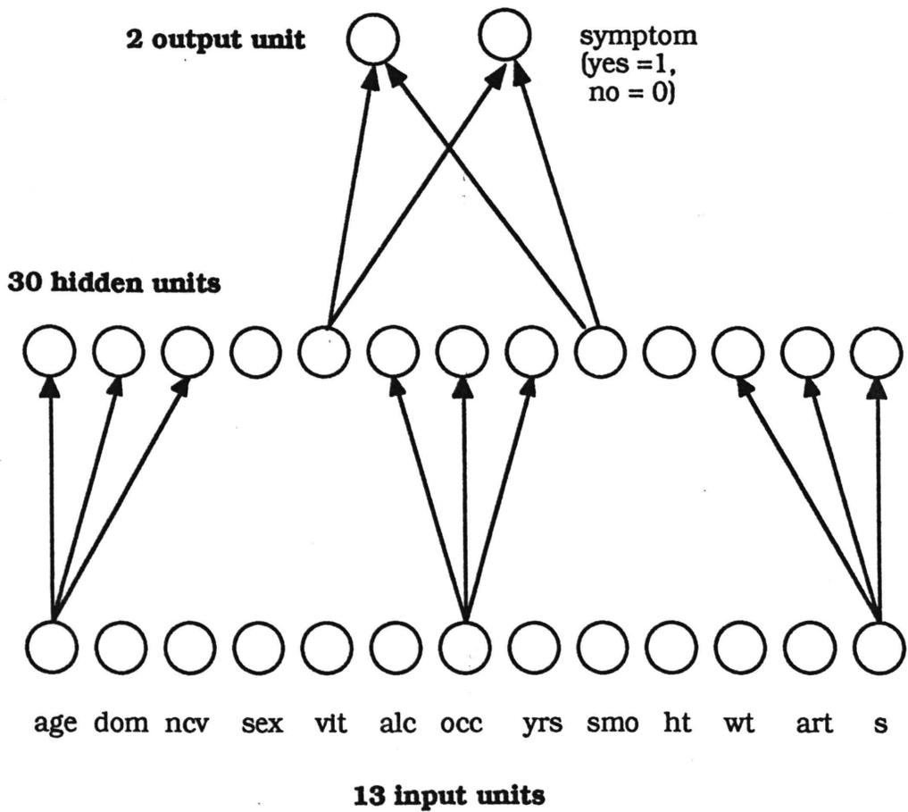
Figure 5.5 Layout of Network for Symptom Classification
