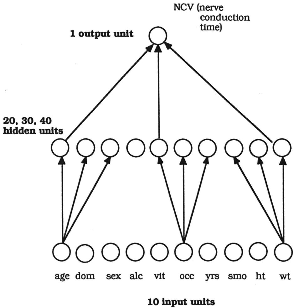
Figure 5.2 Layout of Network for NCV Approximation with Data Set A
