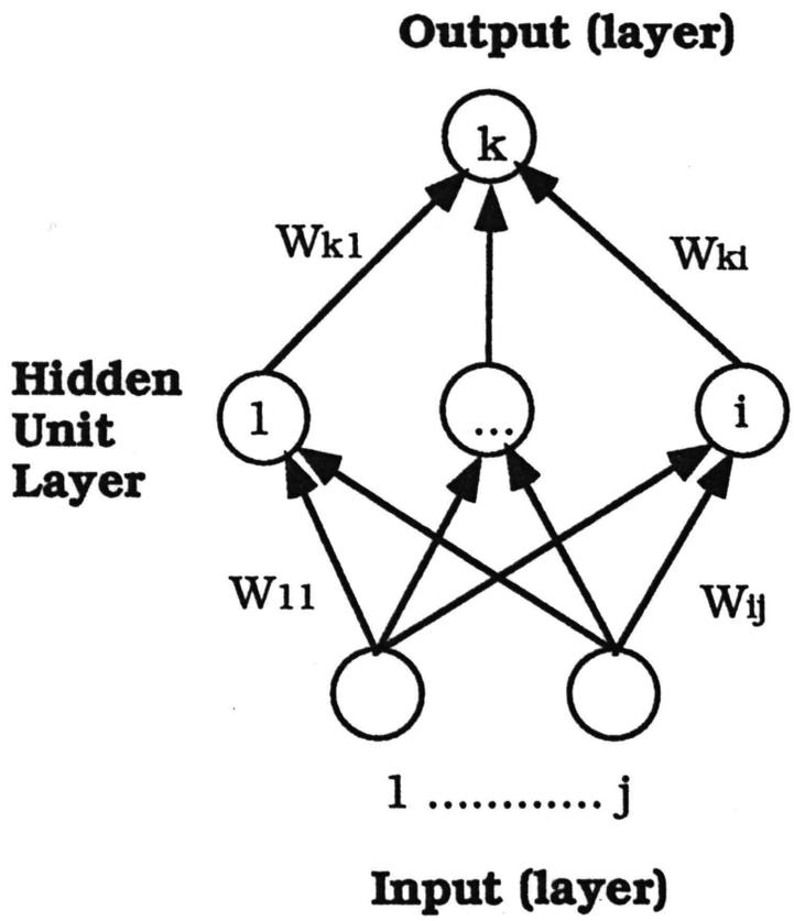
Figure 5.1 Back Propagation Network
