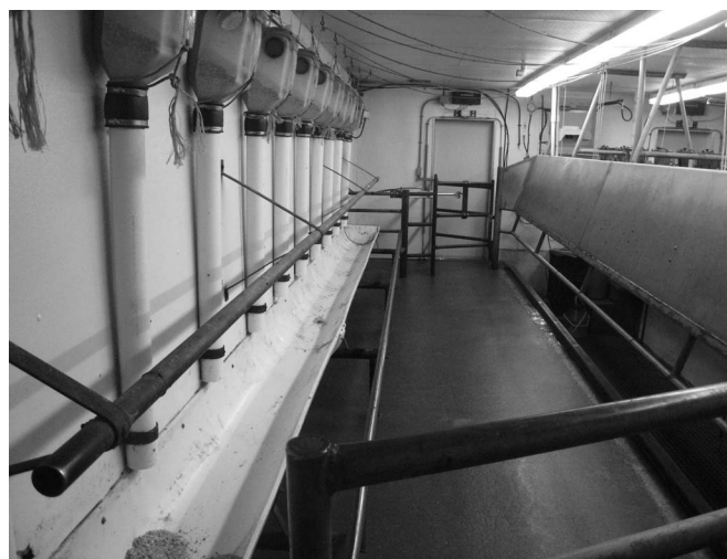
Figure 1. Swing parabone dairy parlors are designed to promote production efficiency by emphasizing cow comfort, cow movement and efficient use of labor.
