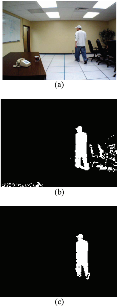
Fig.2: (a) Original image, (b) Silhouette without shadow suppression and (c) Result with shadow suppression
