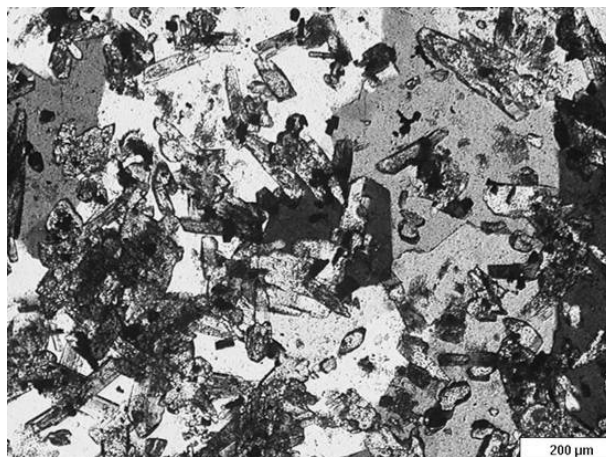
Figure 1. Photomicrograph showing typical end-member epidiosite mineralogy (crossed polars). Note the dominance of anhedral quartz and euhedral epidote, and the lack of preservation of igneous texture.
